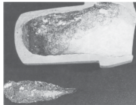
Fig. 8. Melting alloys for the conventional technique by induction, in a silica crucible is difficult because of the oxide layer formed at the surface which leads to scoria formation
